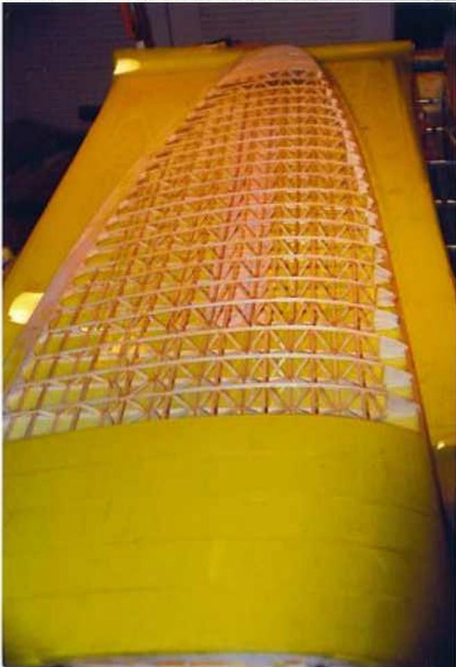
Don says; the Valkyrie should really be recovered after repairing the wing spars. Note that those spars are small, 1/8sq. spruce, but there are so many glue joints that the whole wing should be checked for solid joints as I did years ago when I recovered the wing -- as should the tail. The best covering would be SAM Span [polyspan] because the dope increases
