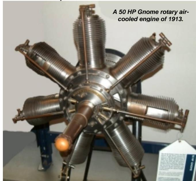
**A 50 HP Gnome rotary air-cooled engine of 1913.**
