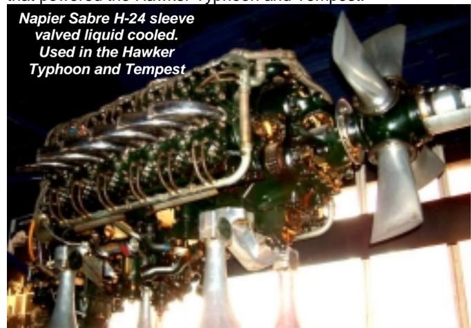
**Napier Sabre H-24 sleeve valved liquid cooled. Used in the Hawker Typhoon and Tempest**
