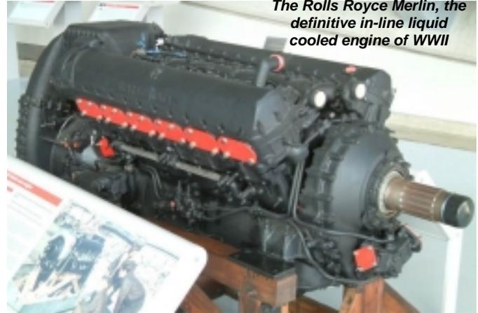
**The Rolls Royce Merlin, the definitive in-line liquid cooled engine of WWII**
