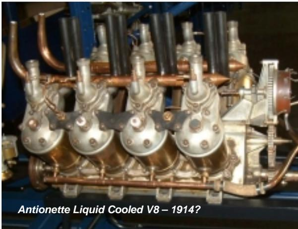
Eventually, designers discovered that the inertia in the gas, which has to very quickly enter and exhaust from the cylinder, needed to be encouraged to leave early. So mechanical control of both inlet and exhaust valves incorporating early opening was required.
