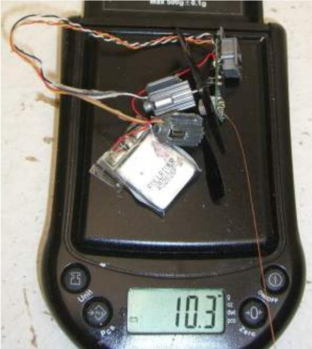
The Air Hog propulsion system and control hardware weighs 10.3 grams and guess what, the battery is ok. I don't know what the problem was but the system seems to work ok now.
