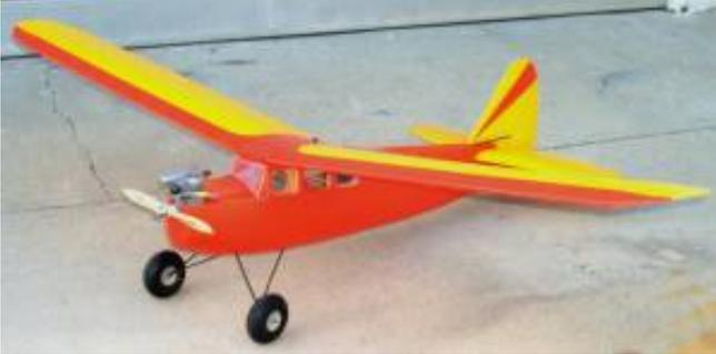
The engine was a Forster 99 and the RC equipment consisted of a single tube circuit mounted by rubber bands and a rubber driven rudder escapement.
