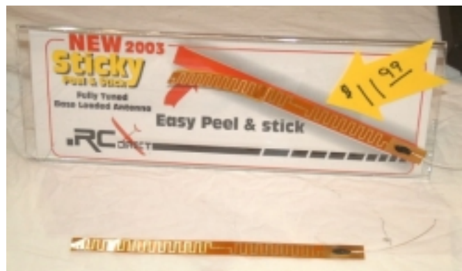
They can be stuck to the surface and connected to the receiver via a short piece of wire and connector.
