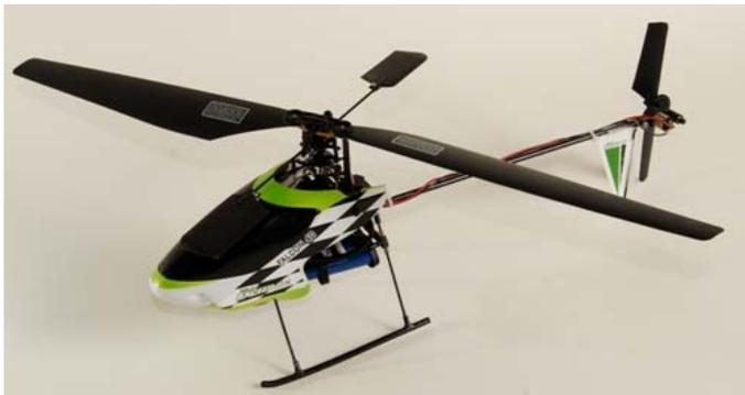
Often the next step from coaxial helicopters, a fixed pitch helicopter has a single set of main blades that are at a fixed angle of attack accompanied by a fly bar with two smaller paddles. The paddles receive the bulk of the cyclic (elevator and aileron to airplane folks) controls and there is a mixing
