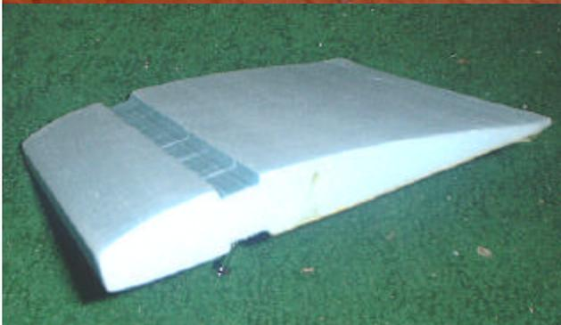
Grooves for spars, etc. are best made after the initial cut. Dick has used a homemade fixture with a short loop of music wire bent to the shape of the desired groove, powered by the same battery charger, to cut spar grooves.
