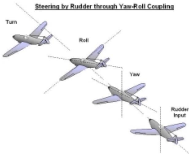
In general, just a few degrees of dihedral are sufficient for adequate roll stability, but to use rudder plus dihedral for roll control generally requires much more dihedral. In my experience, a general rule of thumb for adequate roll control in a typical sport model is at least about 8 degrees of equivalent dihedral per side.
