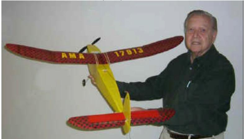
Mick Harris showed a 1936 Fairley Wakefield, an original rubber model converted to electric. One unique feature of this plane is an all flying stabilizer rather than a separate elevator.
