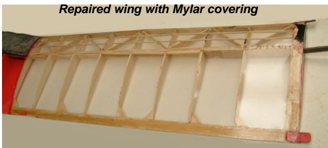
Repaired wing with Mylar covering
