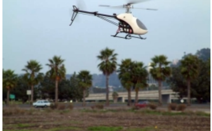
Joker helicopter with large outrunner motor on 32 2400 mah cells
