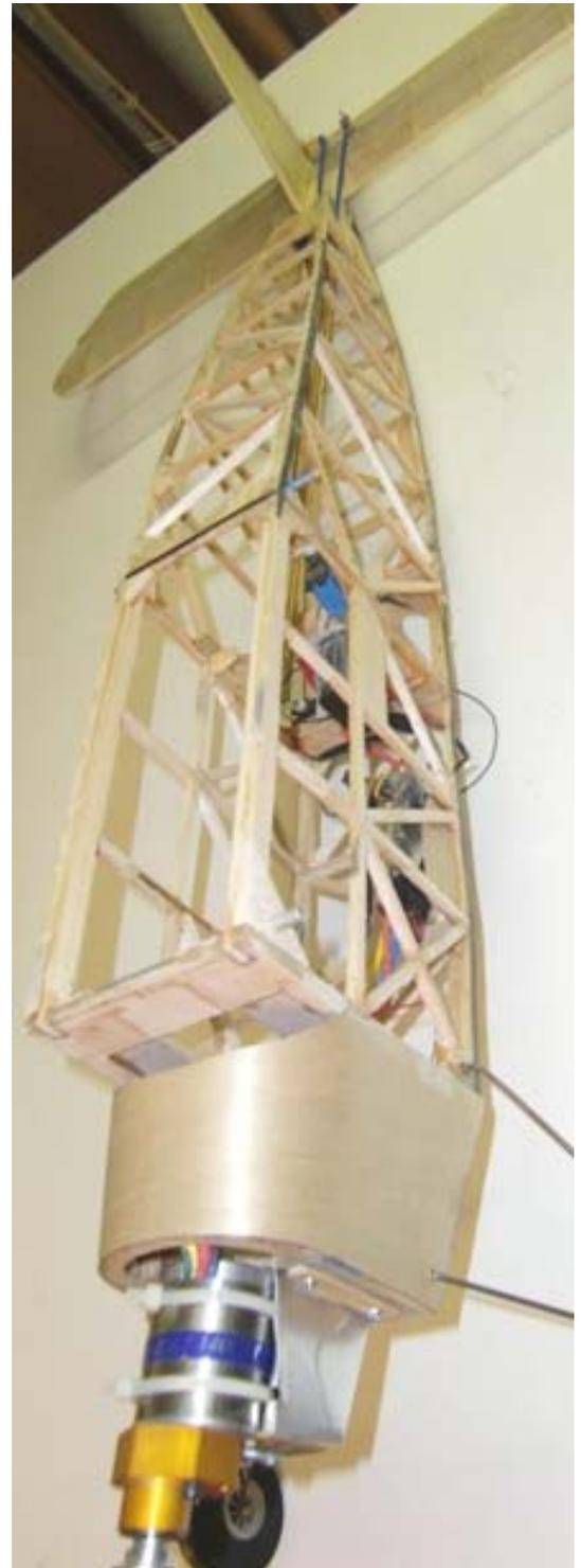
Hammered out the motor mount and fixed the motor. It had been struck from behind by the battery and that dislodged the aft cover and jammed the armature. Just tapped it out and it is as free as ever. My oldest Aveox, nine years old. Holy cow, Frankenstein II, just like last year with the Trenton Terror that stuck in the tree at Pride Day. Now if I can just borrow my covering iron from Drew I can have this ready for this year's Pride Day.
