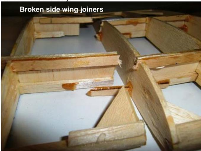
The failure started in the aft spar lower element.
