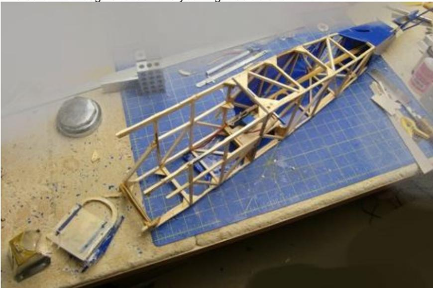
Oops, need to make a completely new forward bulkhead and reinforce the upper wing mount.
