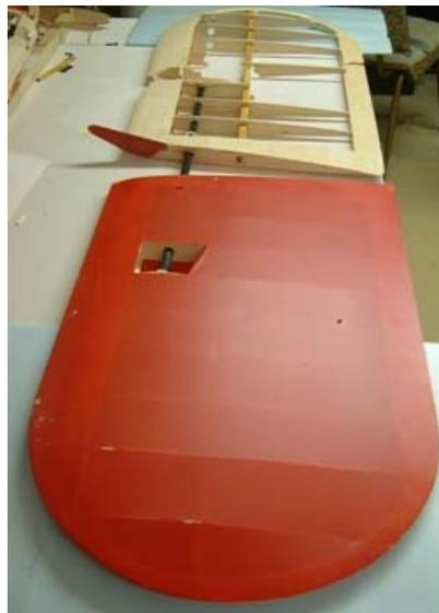
The LH horizontal had departed the aircraft with a failure of the pivot/spar graphite tube flush with the root rib. The other side, the damaged part, remained attached to the aircraft through the pivot/spar remaining half inserted into its socket in the fuselage and the pitch horn attachment to the servo. It had damage in a line diagonally across from front to back; severing the leading edge, trailing edge and the spar.
