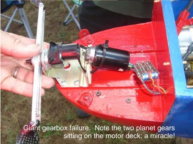
Giant gearbox failure. Note the two planet gears sitting on the motor deck; a miracle!
