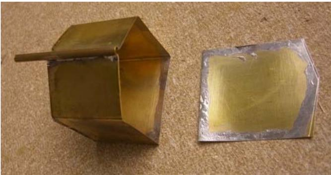
The components are tinned with solder at the location of the joints then soldered together. The vent tube holes are punched into the surface so as to provide a collar to make the joint stronger. Finally the tank is leak and volume tested.
