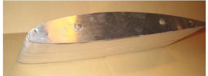
I worked on the airfoil. Used a Boeing 106 airfoil. The profile looked like a good trainer shape. I used your instructions. I cut out two sheets of 1/4" regular plywood alone with two pieces of tin. Sandwiched them, and fastened them with brads. Then cut to shape, sanded and drilled two quarter inch holes through them. After which, I separated the stack and glued a piece of tin to each plywood airfoil.
