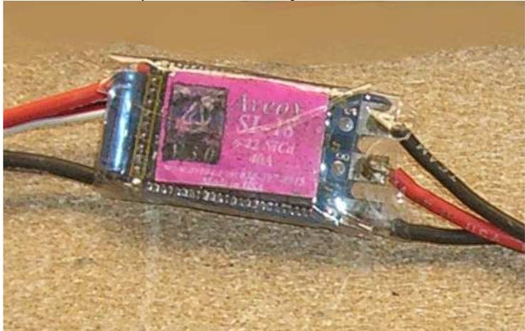
To my horror I discovered that the solder holding the components to the mother board had melted, running between connections in places. What to do? Can this be salvaged? So the first thing I did was to clean up the solder traces between junctions then thinking about the smoke it seemed like it was local to one or two components so I carefully brought the throttle up again and verified that was the case. Now what?
