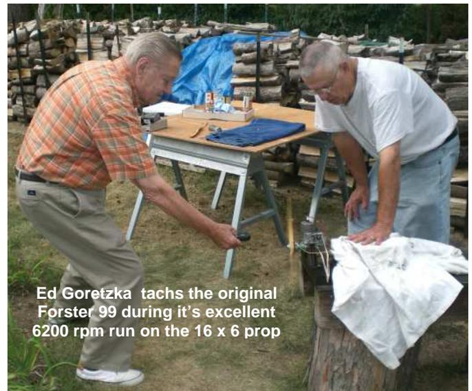
Ed Goretzka tachs the original Forster 99 during it's excellent 6200 rpm run on the 16 x 6 prop
