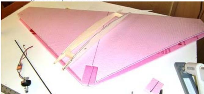
I glued the ribs to the lower surface using hot melt glue. Then I glued the top half to the ribs also with hot melt; work fast!
